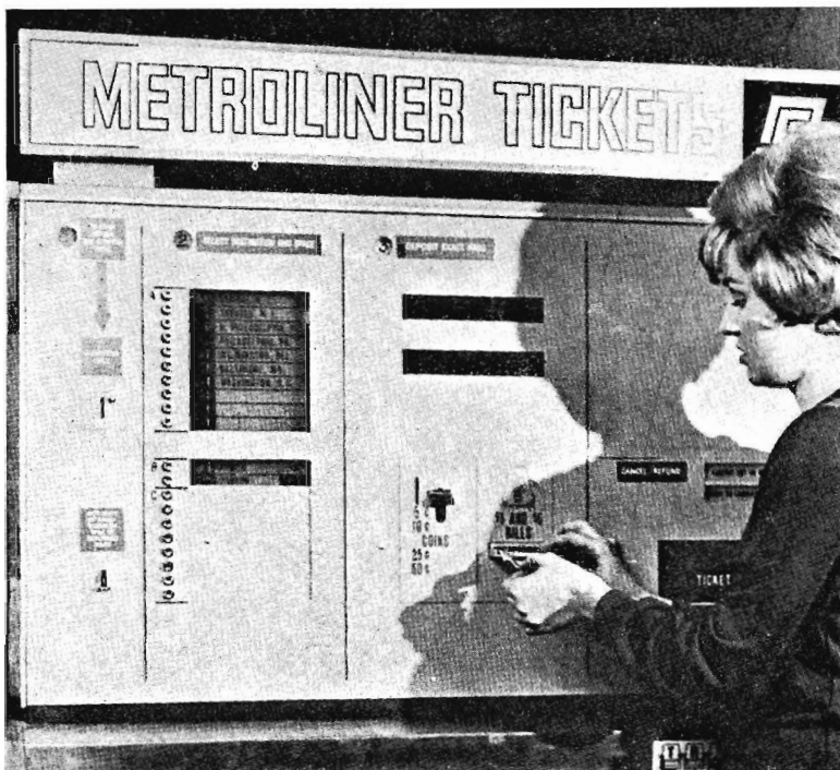
The Metroliner vending machines, thought to be unique in the world, sell tickets only for the next departure. By dropping a 25c piece into the inquiry slot, a passenger can then select the type of accommodation required. The machine indicates if the space is available and the fare. After the passenger deposits the fare, the ticket is printed and dispensed by the machine. The machine accepts coins and $1 and $5 notes.
