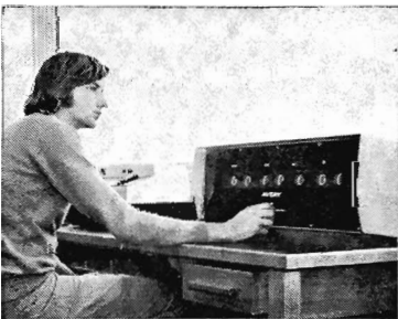
Inside the operator's cabin, the weights of each axle and a total for each wagon are shown on the digital indicator. The machine at left (a Keinzle printer) prints the weights.
