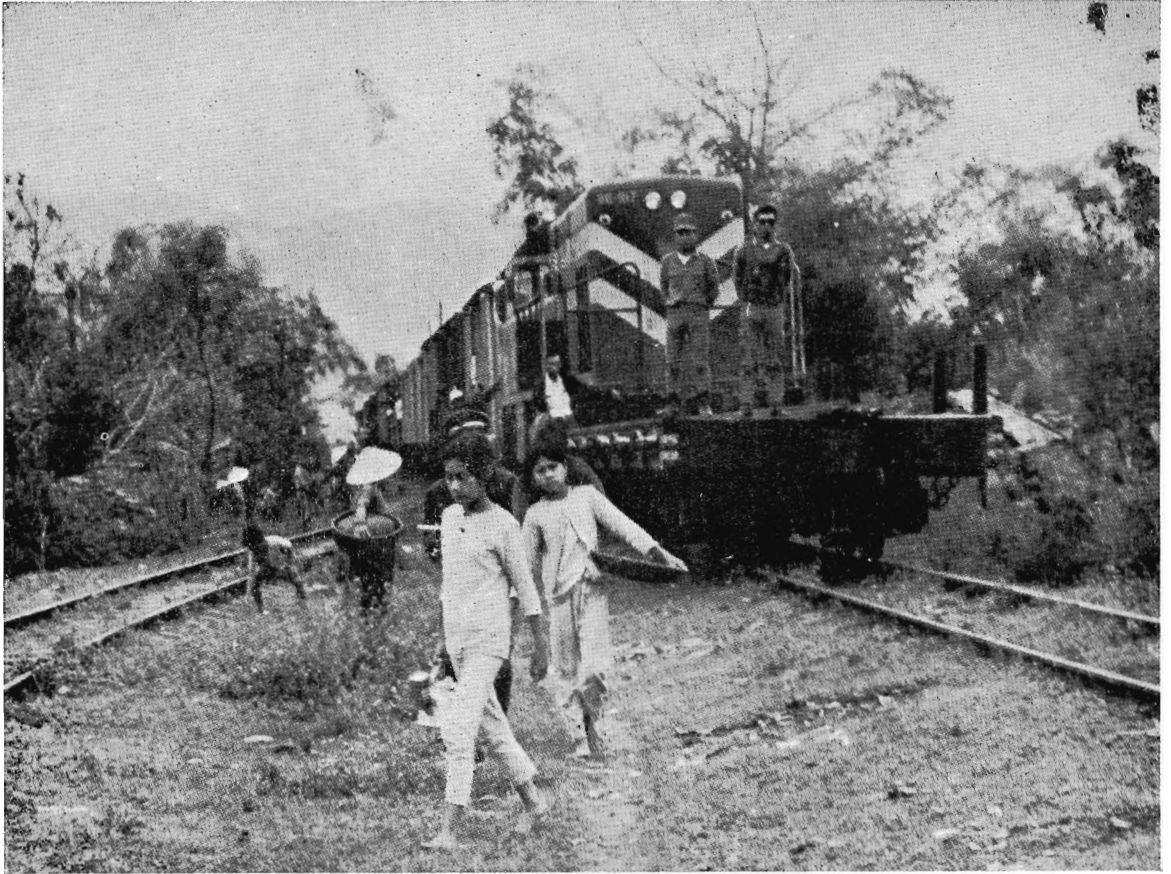
South Vietnamese Army soldiers ride a flatcar preceding the Da Nang-Hue train. The flatcar detonates pressure mines in the train's path. Enemy attacks often follow.
