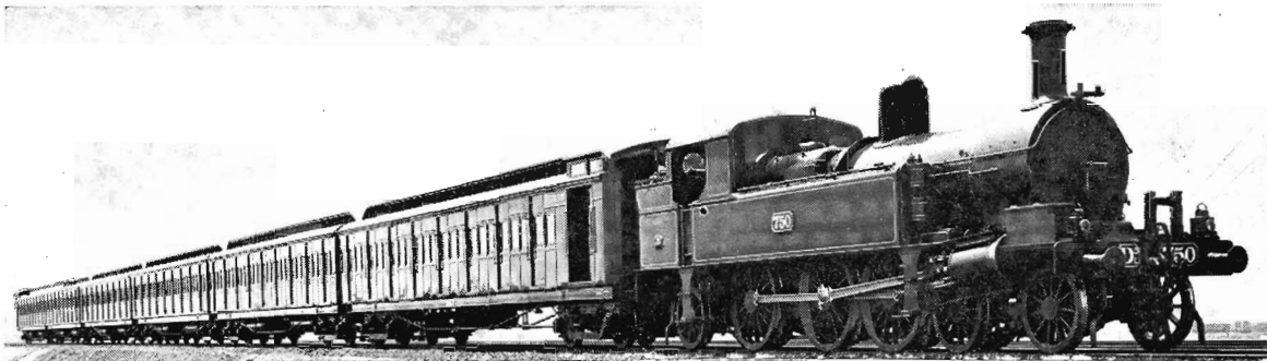
Melbourne's most common metropolitan stock, the Tait trains, were introduced when services were steam-hauled.
