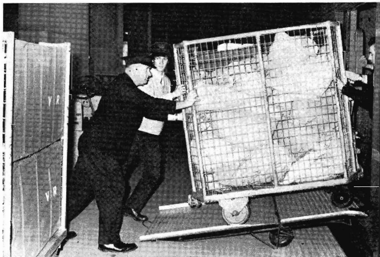
Parcels Foreman Peter McArdle (left) helps unload a container trolley. Despite their heavy appearance, they weigh the same as existing trollies, and are easily handled and manoeuvred. Trolley at far left shows the blind arrangement.
