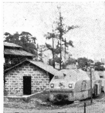
Wickhams , small diesel-powered armoured cars, are used to protect some trains, especially those with military cargoes.
